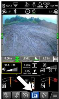
Illustration 59 g07800722 Select E-Fence icon on the monitor display.
