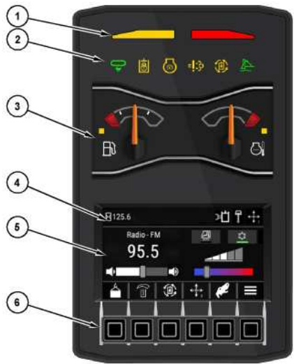
Illustration 1 g06347988 (1) Action Lamps (2) Status Indicator Area (3) Gauge Area (4) Status Information Area (5) Cabin Status Area (6) Navigation Buttons
