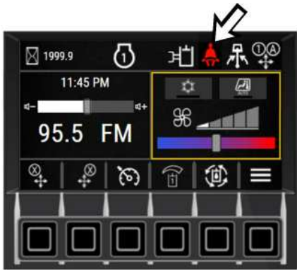
Illustration 94 Seat Belt Indicator in Monitor
