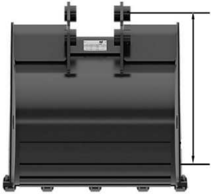
Illustration 38 g07268403 Rear view of bucket G-Q Dimension of bucket Refer to Illustration 38 to measure the G-Q dimension of bucket.
