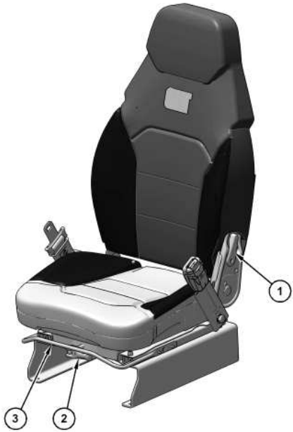
Illustration 2 g06276793 (1) Recline Lever (2) Weight Adjustment Lever (or knob) (3) Seat Fore and Aft Lever
