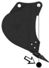
Illustration 35 g07187210 Incorrect way to position the plumb line with bucket
