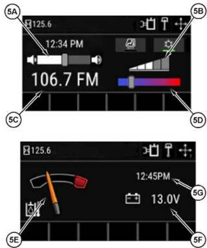
Illustration 5 g06390246 View of status area With and without Radio and HVAC installed
