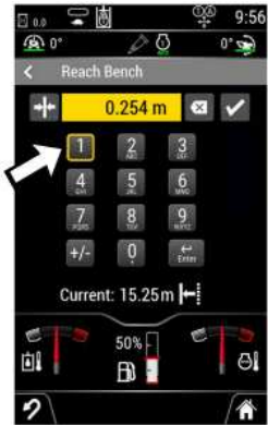
Illustration 49 "Reach Bench" menu in monitor Ok
