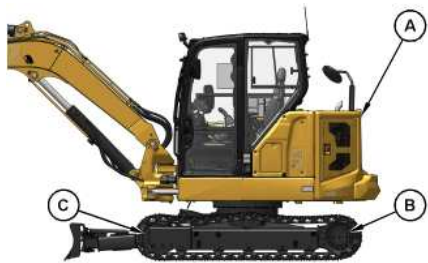
Illustration 8 g06349484 Position for normal travel (A) Rear of machine (B) Final drive (C) Idler
