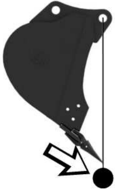
Illustration 36 g07187238 Correct way to position the plumb line with bucket
