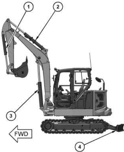
Illustration 1 g06702275 (1) Work tool cylinder (2) Stick cylinder (3) Boom cylinder (4) Blade
