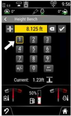
Illustration 47 g06743435 "Height Bench" menu in monitor
