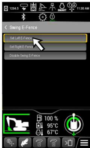
Illustration 58 g06751788 "Swing E-Fence" menu in monitor
