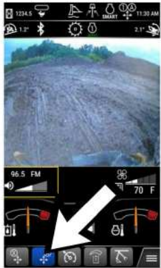
Illustration 17 g07800708 Stick Steer Pattern changer
