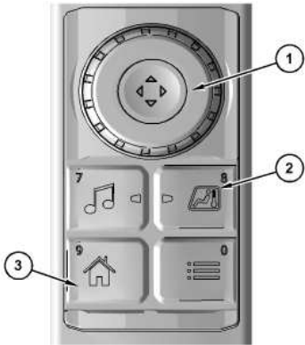
Illustration 1 g06348804 (1) Jog dial (2) Heating and air conditioning button (3) Home button
