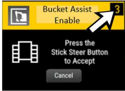
Illustration 68 g07800740 A pop-up window will appear in the monitor display with a timer for 10 seconds within which the bucket assist operation needs to be enabled.
