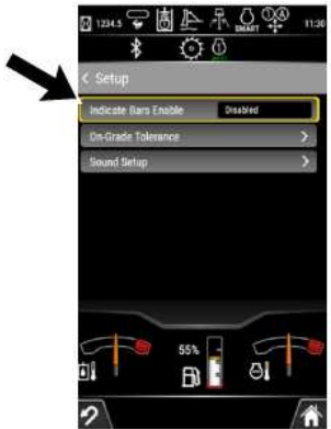
Illustration 57 g07600835 "Setup" menu in monitor
