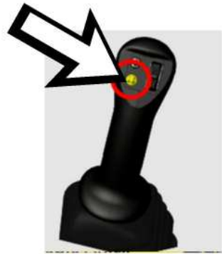
Illustration 69 g07800595 Button on left side joystick Press the button on left joystick to enable the operation. Refer to Illustration 69 for more information. If the operator did not press the button on left joystick to enable the bucket assist within 10 seconds, the operation will fail and return back to the unlock request screen.
