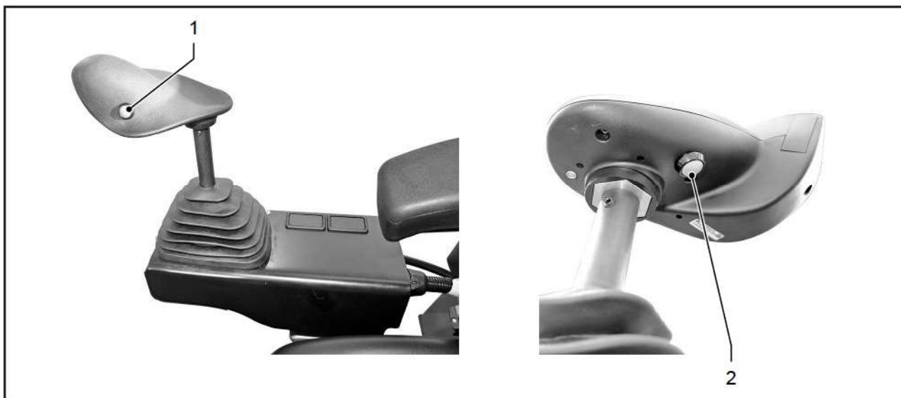
[1] Dynamic compaction system switch
