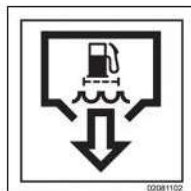
Drain outlet for fuel filter water sump
