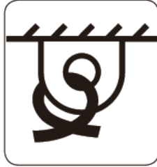
15. No.0881031549 Tie down point
