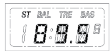
Frequency display (Automatic seeking is stopped. When stereo sound is received, "ST" pict turns on)
