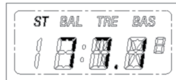
Frequency display (Automatic seeking is stopped. When stereo sound is received, "ST" pict turns on)
