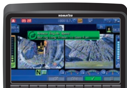
Eco-gauge, Eco guidance and fuel consumption gauge
