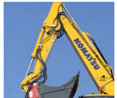
New HCU piping layout with a unified design for all arm lengths
