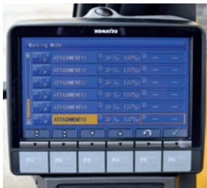
Komatsu Integrated Attachment Control (KIAC) for up to 15 tool presets for oil flow and pressure
