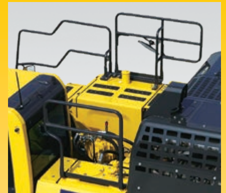
Hand rails and anti-slip plates
