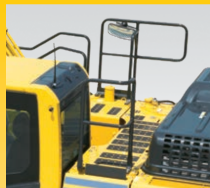
Hand rails and anti-slip plates
