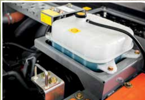
The expansion tank prevents engine parts from overheating.
