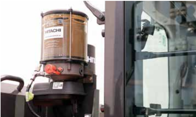
Optional auto-greasing system saves time.
