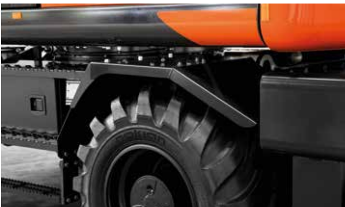
Fenders on the undercarriage protect the upper structure and lights from dirt, keeping the machine clean.
