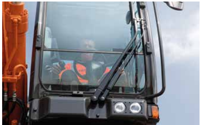
Wider wiper design provides greater visibility.
