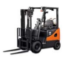
D15S / D18S-5 & D20SC-5 G15S / G18S-5 & G20SC-5 1,500kg 1,750kg 2,000kg Diesel, LP, Gas, Pneumatic Tire
