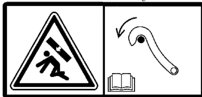
Figure 8: Counterweight crushing hazard, use lock lever (6)
