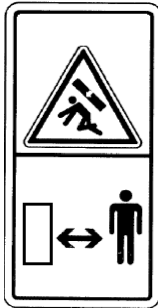
Figure 7: Counterweight crushing hazard and pinch point (5)
