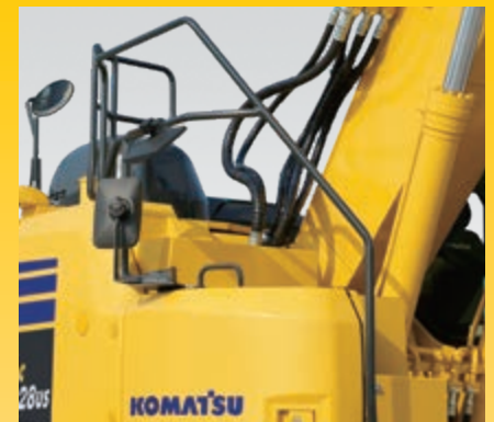
Hand rails and anti-slip plates
