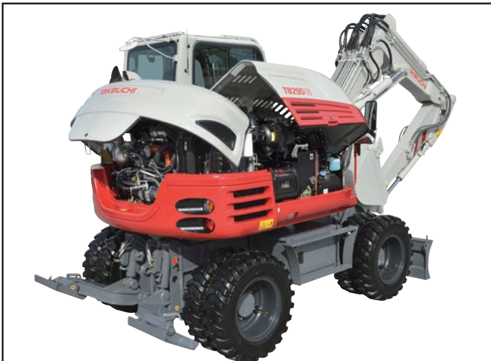
Large Lockable Service Hoods Provide Ground Level Access
