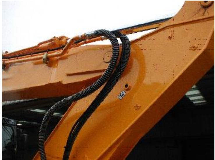
Pipe routing from dipper to boom. Cable tie to existing hose
