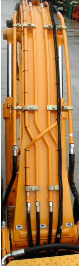
Cable tie the two longest hydraulic pipes to existing hydraulic pipes along the boom.
